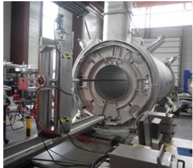
Fig. 3. Warm coil field mapping of the SHMS Dipole at Sigma Phi.
