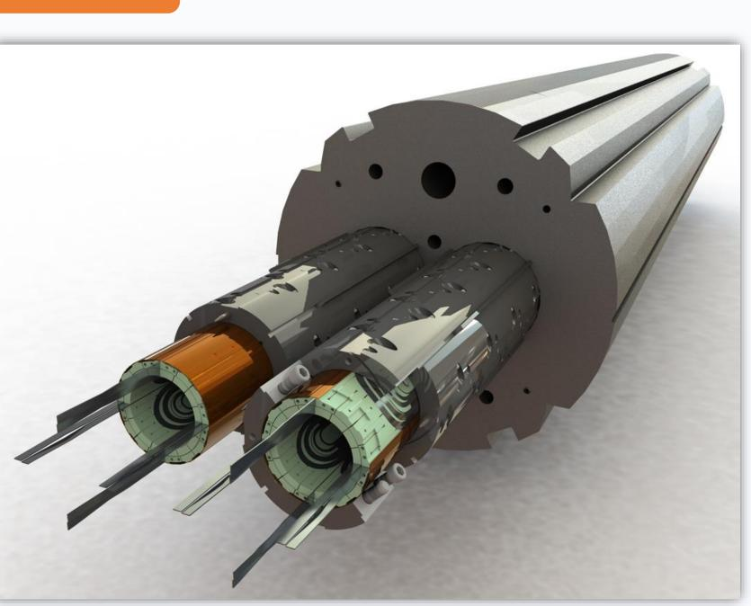
Aluminum collars alf collars assembled aroun the coils with a press Fixation with aluminum bolt & titanium pins
